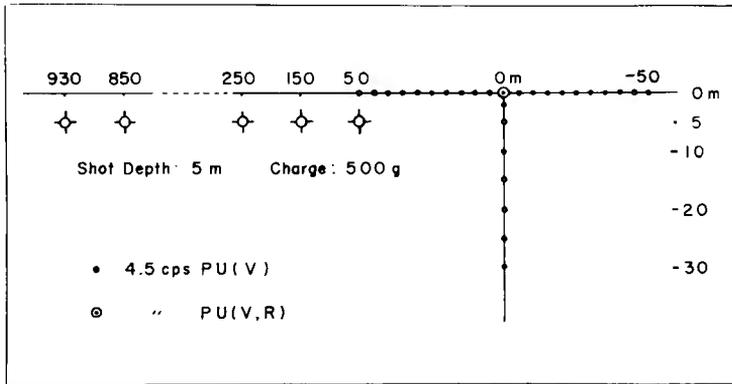
Fig. 1. Spreads of the seismometers and shooting points.
