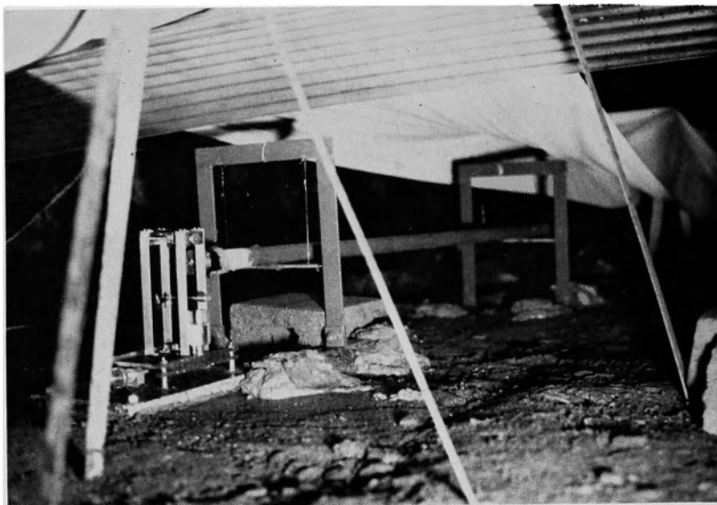
Photo. 4. Amplifier part of the H-59-D type extensometer.
