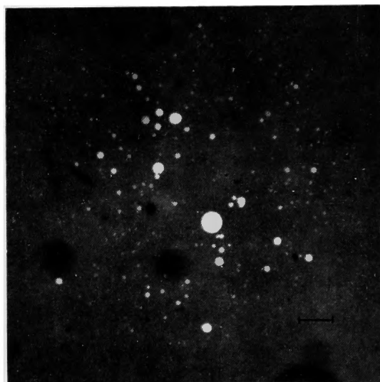
Fig. 6. An example of the halo area on the reagent film provided by the impactor. The line entered indicates 100\mu .
