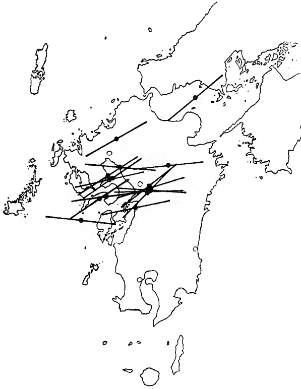
Fig. 6. Direction of the compression axes in the western area of Kyushu Island.
