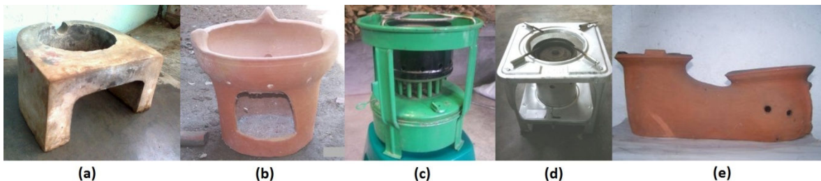
Figure 4.9 Stove types for WBT test (a. wood stove, b. charcoal stove, c. kerosene stove, d. JCS stove, e. improved wood stove-SAE stove)
