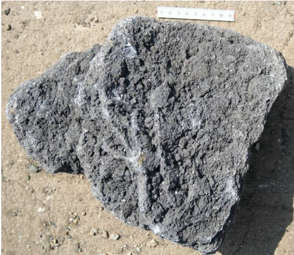
Fig. 5-11. Fraction of SR in the wall side of the kiln.
