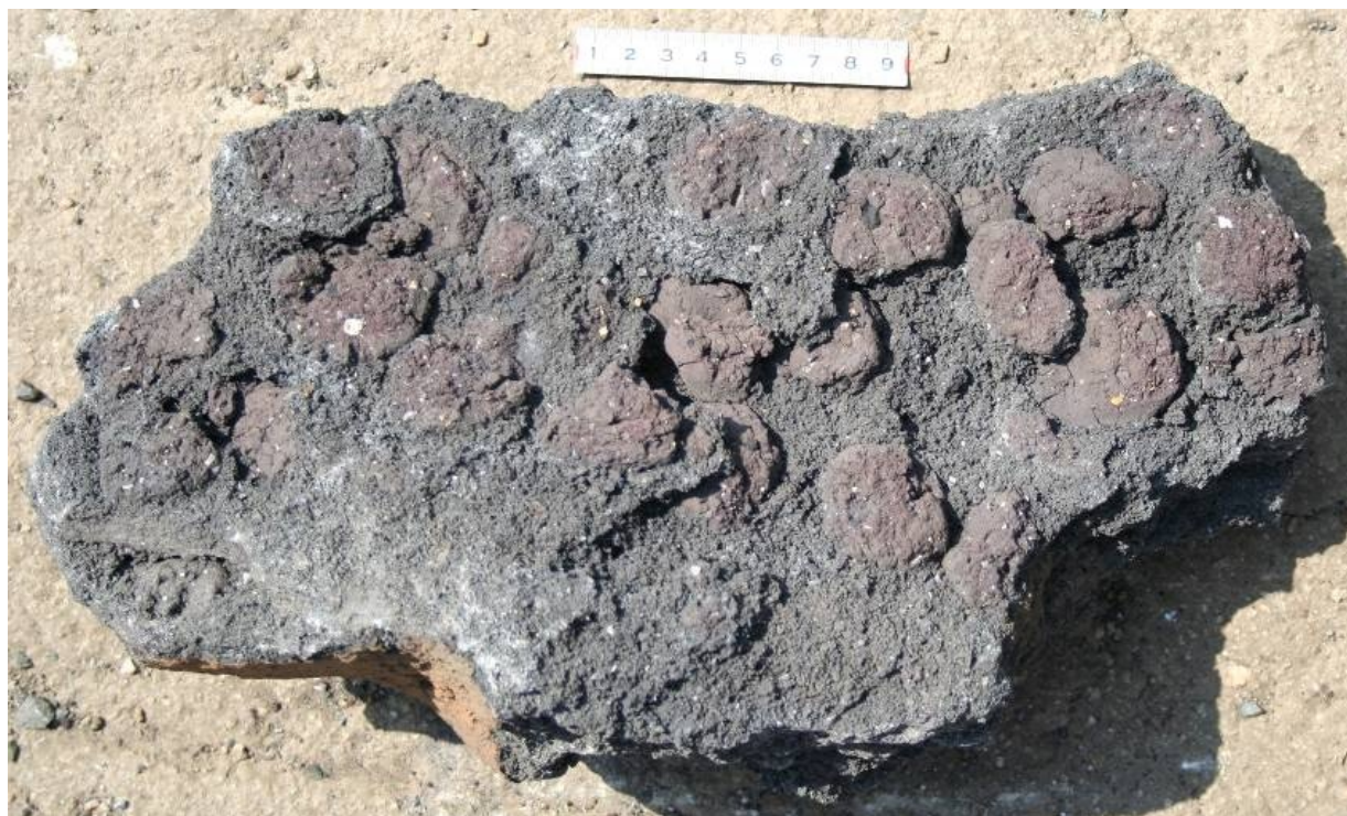
Fig. 5-10. Fraction of SR involving briquettes in the raw materials side of the kiln.
