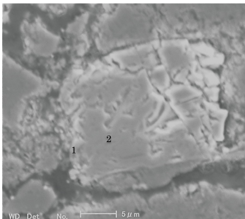
Fig. 2-24. SEM image of spinel in Ore-A at 1050 (1.2A 0 ).
