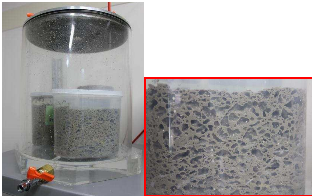
Figure 4.4 Silica sand-bentonite specimens in vacuum tank.
