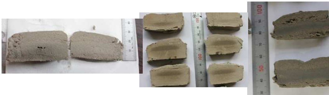
Figure 4.15 Photo of shear zones after shearing: a) SB 20 at 0.1 mm/s until 5 m, b) SB 30 at 1 mm/s until 10 m and c) SB 30 multi-stage test with total displacement of 30 m.
