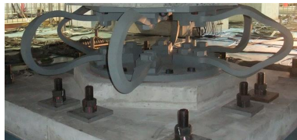
Figure 4.9 U-shaped damper after all shakings
