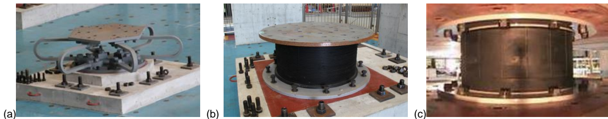
Figure 4.3 Base isolation system: (a) U-shaped steel damper; (b) natural rubber bearing; (c) high damping rubber bearing
