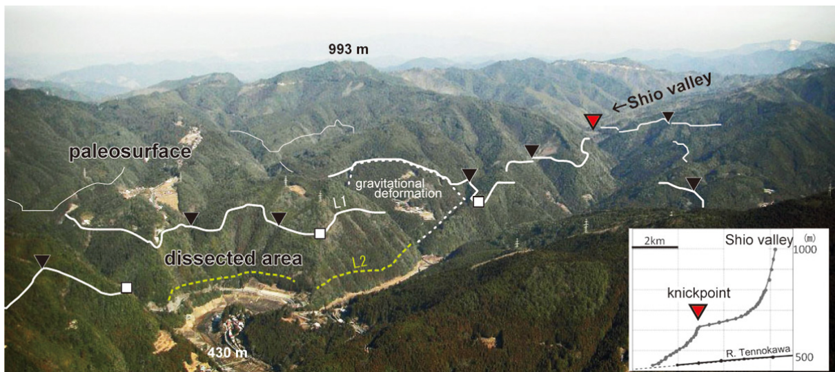
Fig. 2 Oblique view of the landscape in the study area shown in Fig. 1. Sharply-defined upper slope breaks “L1” (white solid lines) are distributed >100 m above the riverbed of the Tennokawa river. L1 divides the study area into two areas; upper paleosurface and lower dissected areas. These slope breaks are sometimes removed by landslides or blurred by gravitational slope deformation. In that case, we traced the outlines of landslide heads as the slope break. A long-river profile of a tributary “Shio valley” is shown in the bottom-right corner as an example. Squares are representative points of slope breaks’ altitudes (Fig. 9). In dissected area, lower slope breaks “L2” (yellow dashed line) are distributed intermittently.
