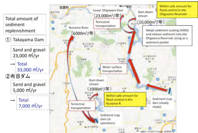
Fig.10 A proposal of sediment augmentation methods for Takayama Dam and Nunome Dam in the Kizu River.
