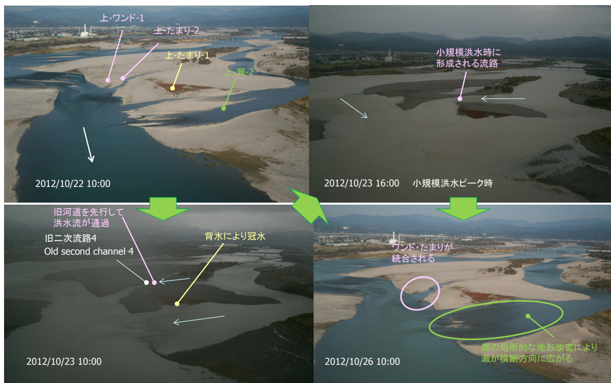
Fig. 7 Flow direction and characteristics of geo-morphological change at the upstream reach in a small size flood event occurred on 23 October 2012.
