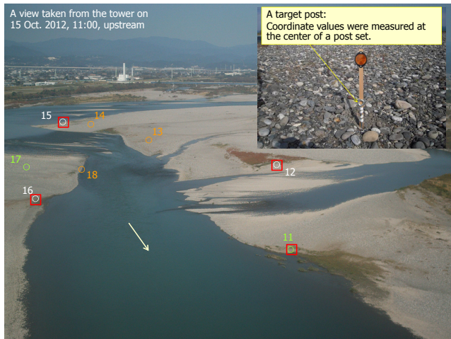
Fig. 14 Data transformed into the ortho data through the photogrammetric method. “○” in the fig. refers to a location where target posts having coordinate values have been set. 2D ortho data were developed based on No. 11, 12, 15, and 16, referred to as “□” in the fig., using a photogrammetric method.
