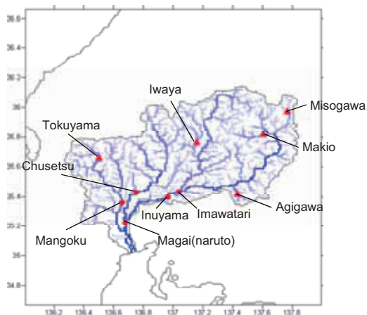
Fig. 1 Channel network, major dam and reference point in the Kiso River System. (▲:Dam;●:Reference point)
