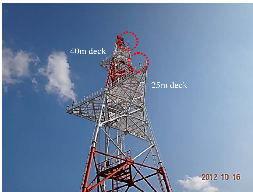
Photo 1 Sonic anemometer-thermometers (denoted by the dotted red circles) on a tower in the Ujigawa Open Laboratory
