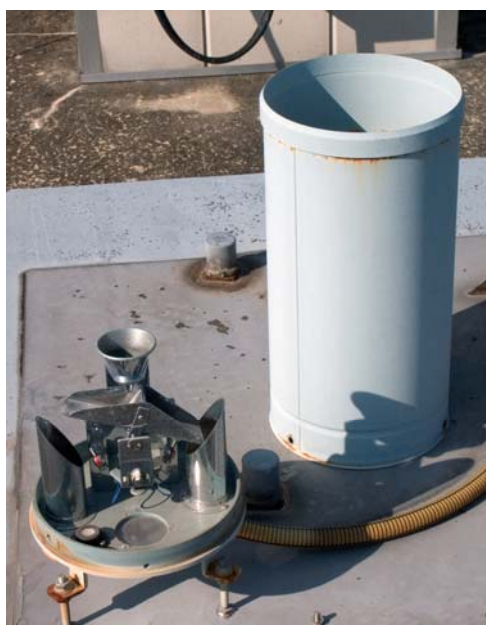
Photo 2 Inside of the rain gauge. The rain water receiver is seesaw-shaped, and it tips for every 0.5mm rainfall. The number of tipping times is counted electrically.
