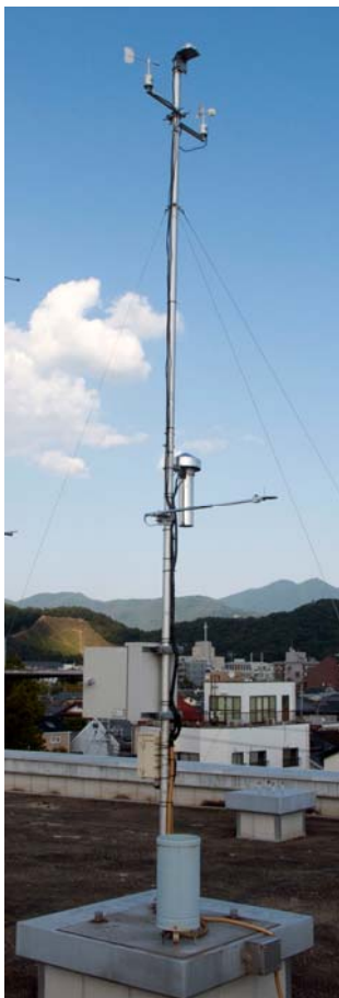
Photo 1 The automatic meteorological observation equipment at Kyoto Prefecture University. The circular cylinder on the base is a rain gauge.
