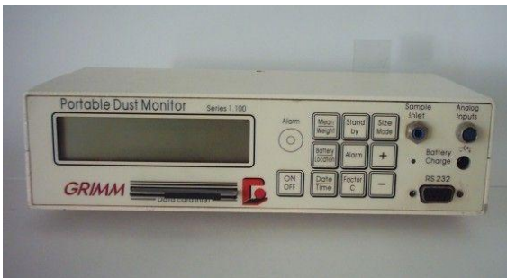
Photo 7 Portable aerosol spectrometer: The instrument gives real time particles in 31 different size channels.
