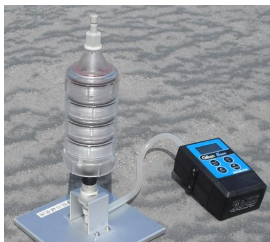
Photo 3 Air-pump and filter folder; Air-pump has 5000cc/min. of maximum suction capacity.
