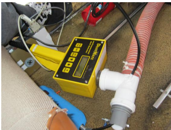
Photo 6 Dust meter: Total, PM10, PM2.5, PM1.0 particles are monitored. Brown tube from the dust meter is connected to the air vent of the plane.
