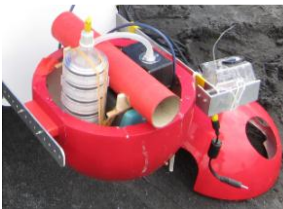
Photo 4 Digital dust meter, filter folder inside wind shelter and small video camera; Wind shelter is attached in the front of UAV
