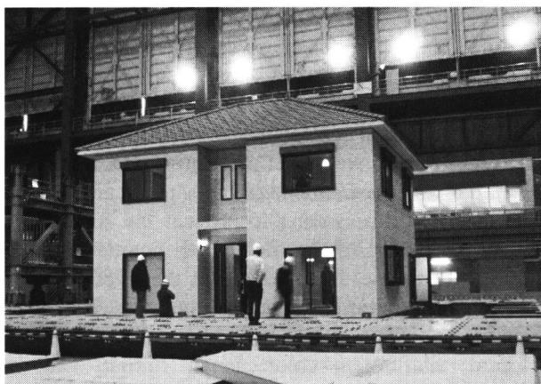
Fig.1. A two-story modern wooden residential house just after the first shaking table test over. Researchers are inspecting damages with a lot of interests (E-defense, Miki, Hyogo prefecture).
