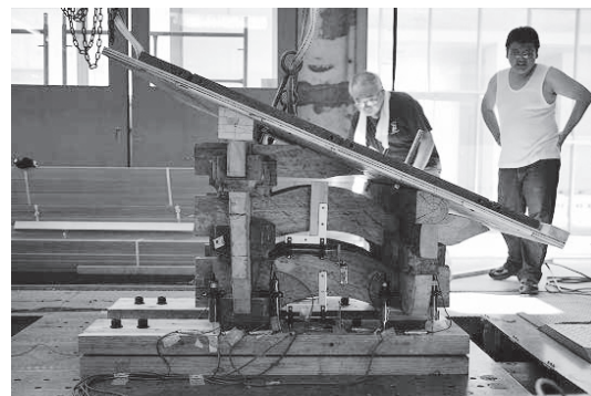
Fig.3 A partial full-scale Kumimono-complex specimen put on the shaking table equipment.
