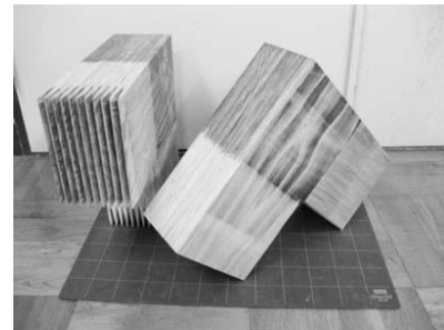
Figure 3. Developed joint method of compressed cross-lapped joint.
