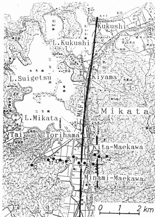
Fig. 36. Location of ELF-MT survey sites across the Mikata fault. Solid lines show the fault lines. MKF: Mikata fault.
