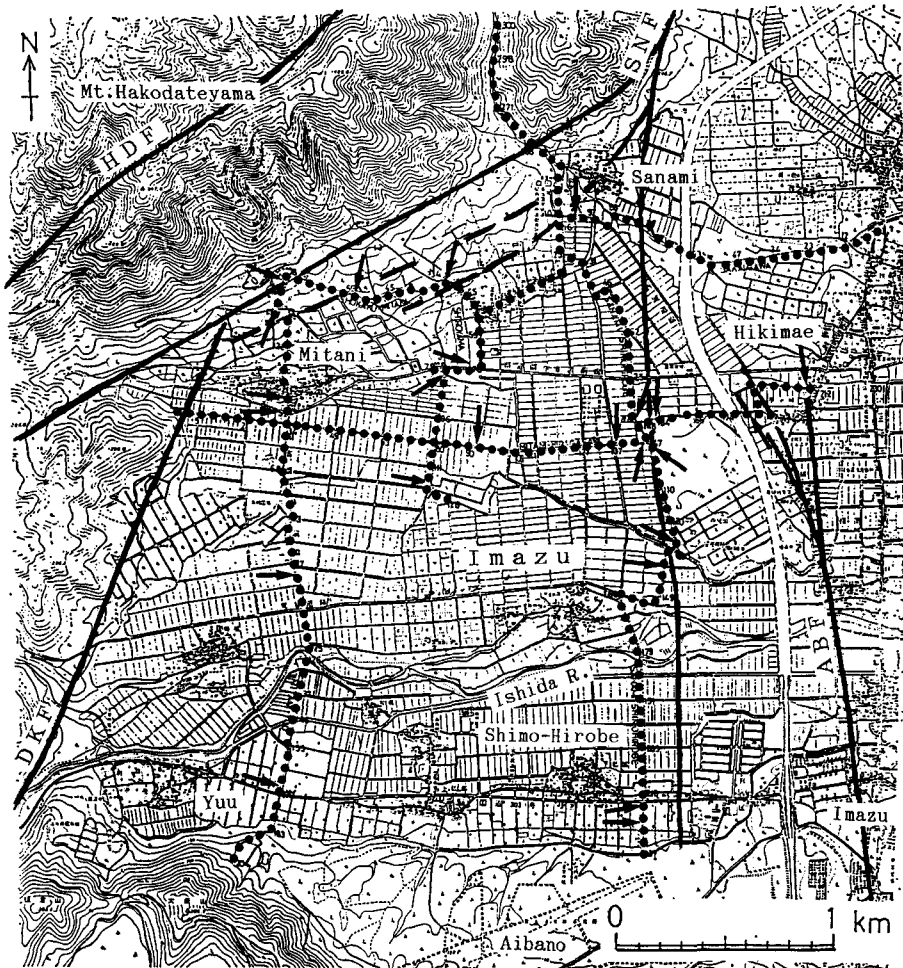
Fig. 34. \gamma -ray survey lines (dotted line) at Imazu. Arrows indicate the points showing high level intensity of \gamma -ray. Solid lines show estimated fault lines. ABF: Aibano fault, SNF: Sanami fault, HDF: Hakodateyama fault, DKF: Dokenyama fault.
