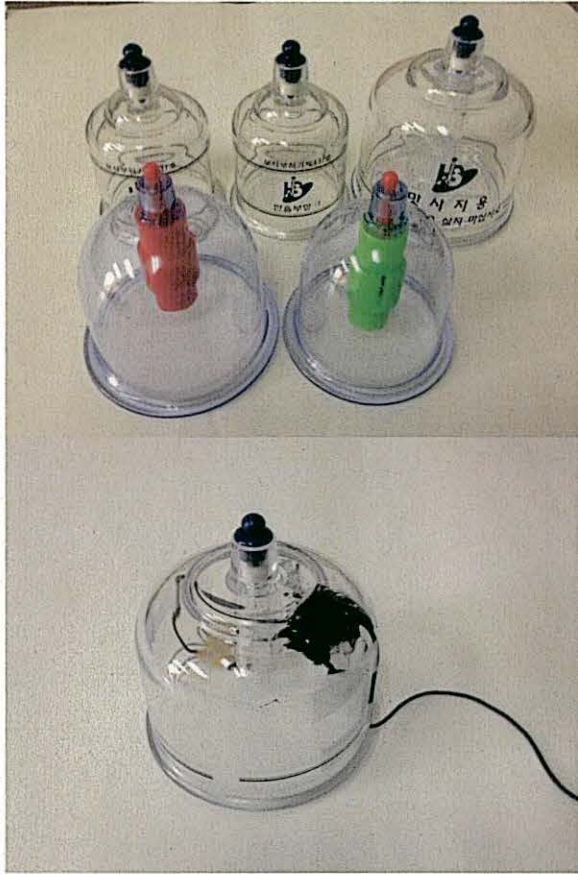
Fig. 1: Acupuncture cups before mounting the phono-transducers (top) and after mounting the microphone (bottom)
