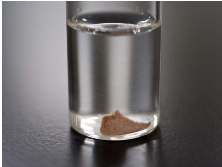
Figure 5.10 The (3-mercaptopropyl)trimethoxysilane–(3-mercaptopropyl)methyldimethoxysilane (3MP, 3MP) marshmallow-like gel adsorbed gold ions on the surface by soaking in an aqueous tetrachloroauric acid solution.
