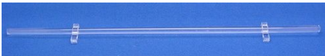
Fig. 6. Obtained fiber preform by extrusion method.
