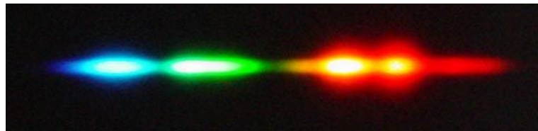
Fig. 1. Amplified spontaneous emission from \text{Pr}^{3+} doped fiber dispersed by prism.
