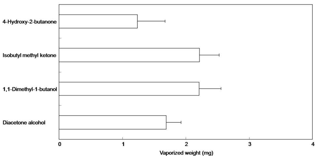
**Fig. 24.** Evaporated weight of diacetone alcohol, 1,1-dimethyl-1-butanol, isobutyl methyl ketone and 4-hydroxy-2-butanone (4 mg/cage) administration in glass cage. Data are shown as the mean values  $\pm$  SEM of 3 trials.
