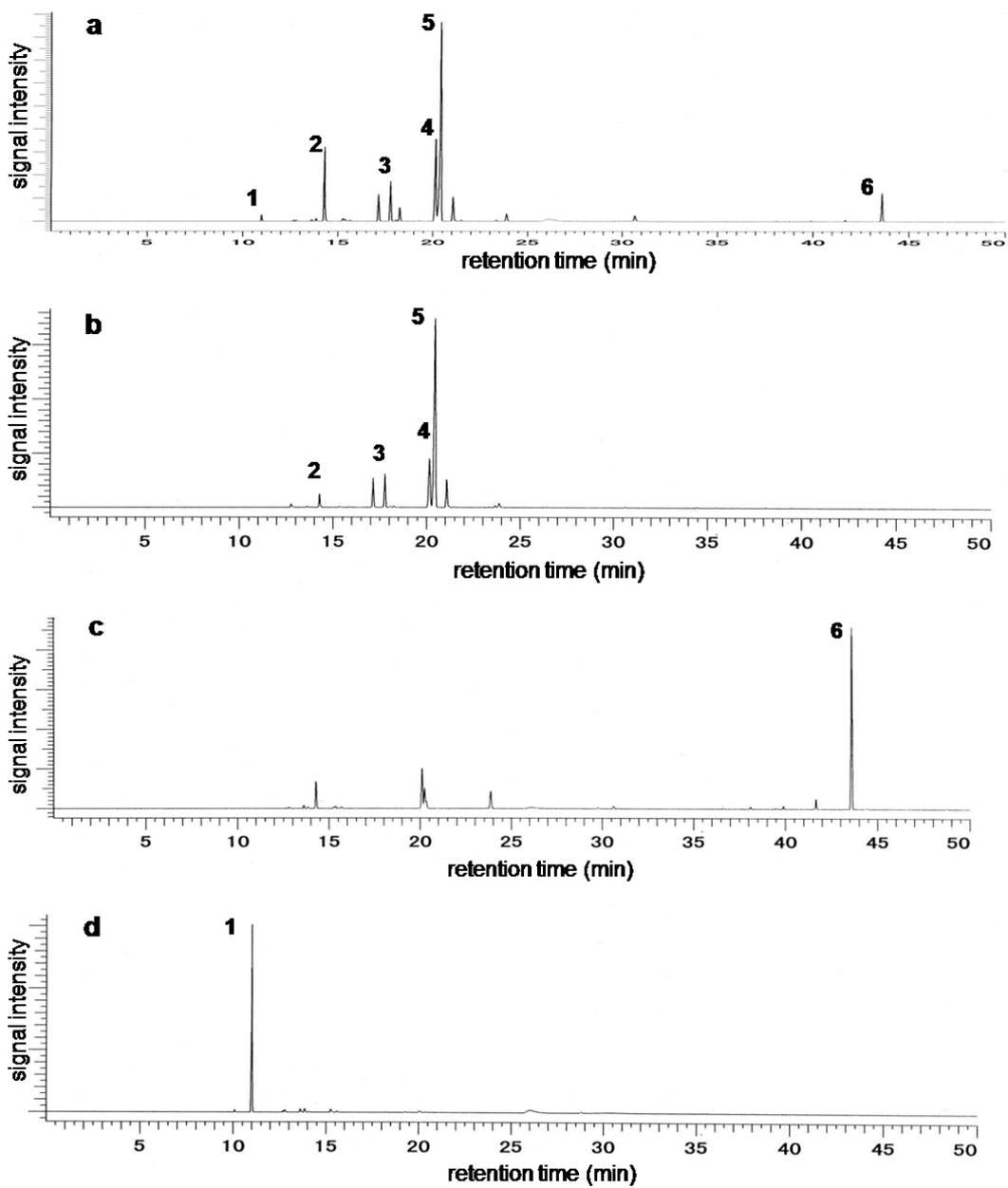
Fig. 4. GC-MS Analysis of *patchouli* extract and fraction 1, 2, or 3 (a, b, c, and d, respectively). Numbered peaks are as follows: 1, diacetone alcohol; 2,  $\beta$ -patchoulene; 3,  $\alpha$ -guaiene; 4,  $\alpha$ -patchoulene; 5, seychellene; 6, patchouli alcohol.
