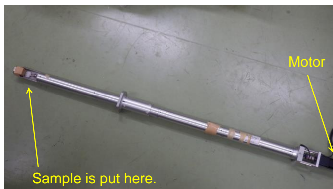
Figure 4.3. Photograph of a rotating unit (KU model \chi 10-3). The suspension of a sample is rotated in a superconducting magnet and subjected to in-situ X-ray diffraction measurement.
