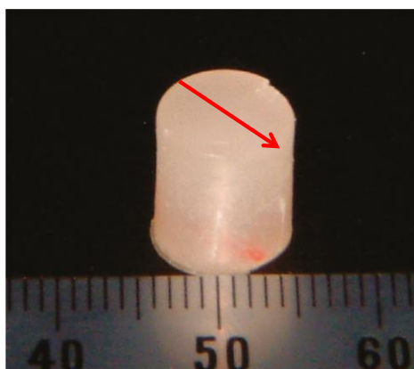
Figure 4.2. Photograph of a magnetically oriented microcrystal array of L-alanine. The crystal is ca. 8 mm in diameter and 10 mm in height. The cylinder axis corresponds to the hard magnetization axis and a red arrow corresponds to the second smallest magnetization axis.
