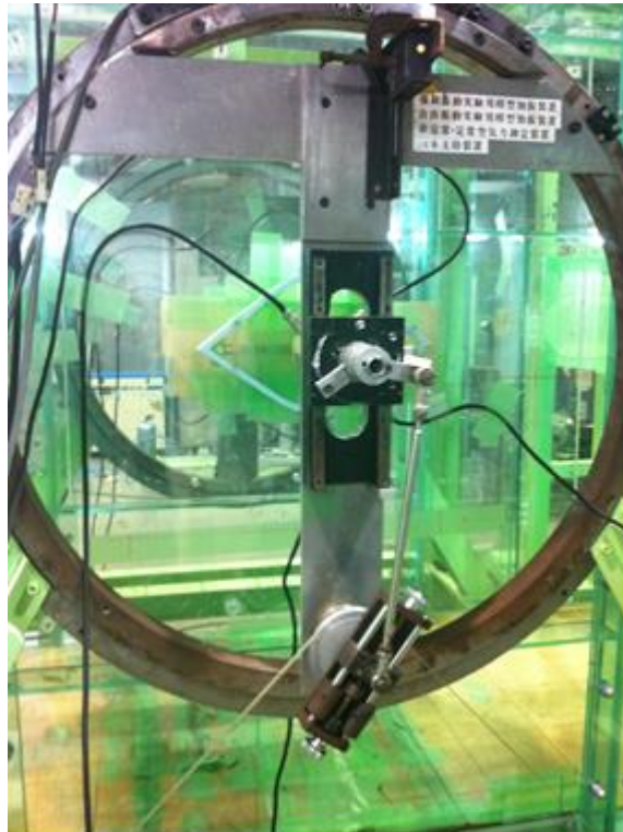
Fig. 5.1 Set up of equipment outside wind tunnel for direct force measurement
