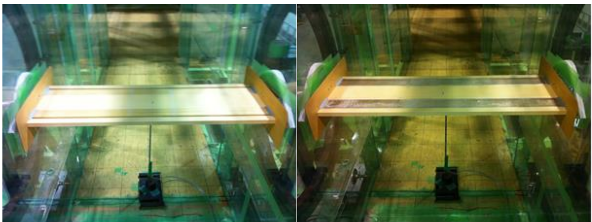
Fig.4.8 Model with double slot (left) and porous cavity (right) during testing
