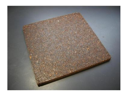
Fig.1. Particleboard bonded with citric acid and sucrose
