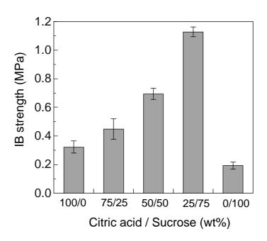
$Fig. 3.\ Effect\ of\ citric\ /\ sucrose\ ratio\ on\ IB\ strength.\ Error\ bars\ indicate\ standard\ deviations$
