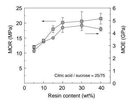
Fig.6. Effects of resin content of citric acid / sucrose on bending properties. Error bars indicate standard deviations
