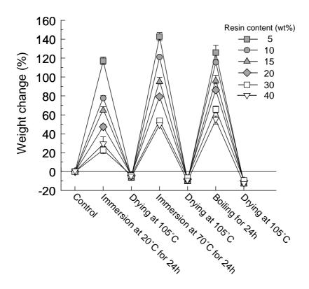
Fig.9. Weight change in a cyclic accelerated aging treatment. Error bars indicate standard deviations
