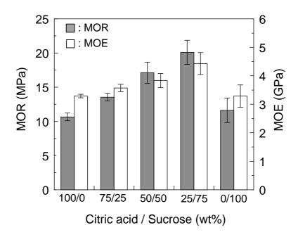
Fig.2. Effects of citric acid / sucrose ratio on bending properties. Error bars indicate standard deviations
