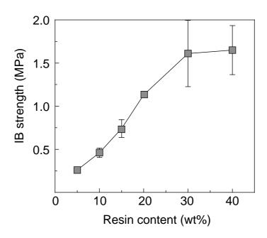
Fig.7. Effects of resin content of citric acid / sucrose on IB strength. Error bars indicate standard deviations
