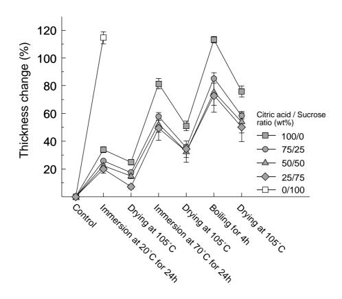
Fig.4. Thickness change in a cyclic accelerated aging treatment. Error bars indicate standard deviations
