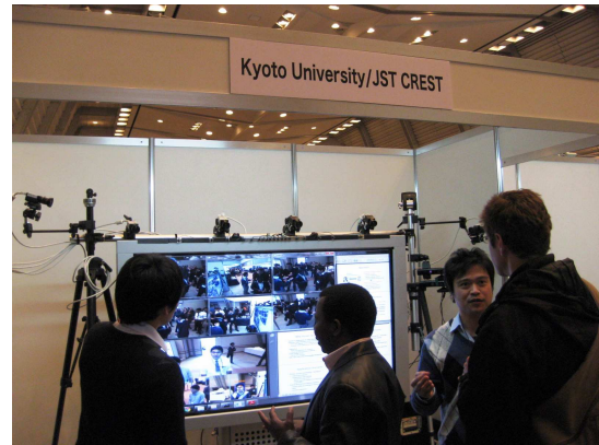
Fig. 1. Smart digital signage for group dynamics analysis showcased at the international conference IEEE ICASSP 2012. The system consists of a large display and multiple sensing devices (e.g. microphone array, HD video cameras, and depth sensors) that perform simultaneous captures. Multimodal interaction dynamics are modeled using hybrid dynamical systems, and interaction level of participants are estimated using audio-visual event statistics.
