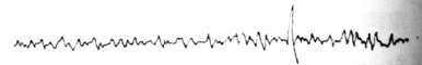
Fig. 12 A sketch of the extreme amplitude which might occur in the running motor-truck.
