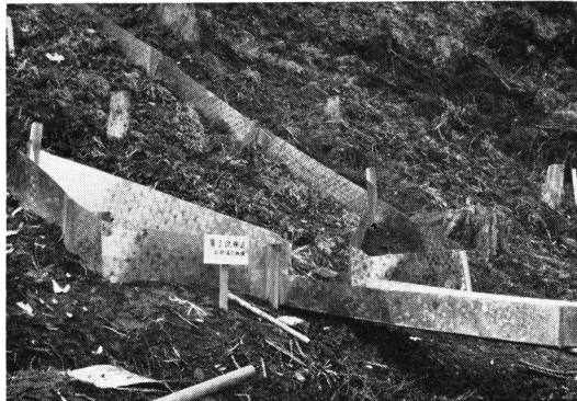
試験枠受器の構造 Structure of the measuring frame for soil erosion.
