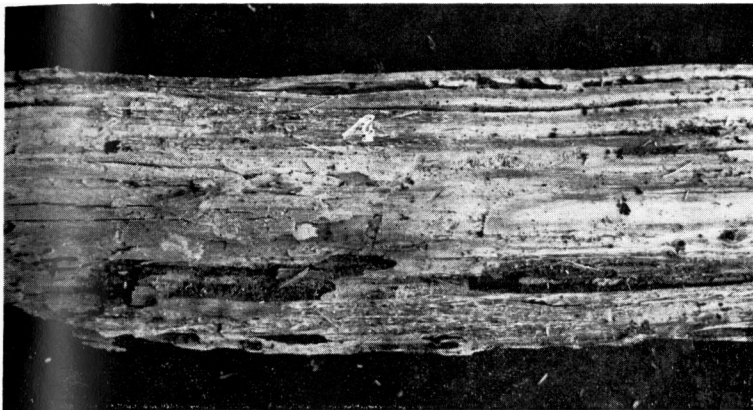
Photo 10 Condition of decay of red pine test stick after two years
