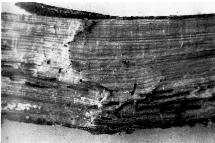
Photo 11 Galleries of bark beetles in test stick of beech
