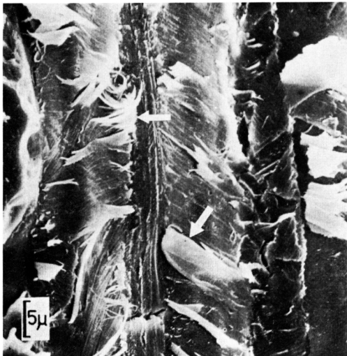
Plate 7. Micrograph of the same surface as shown in Plate 5, showing the replica of wood fibers on which fragments of fiber wall (arrows) were adhered.
