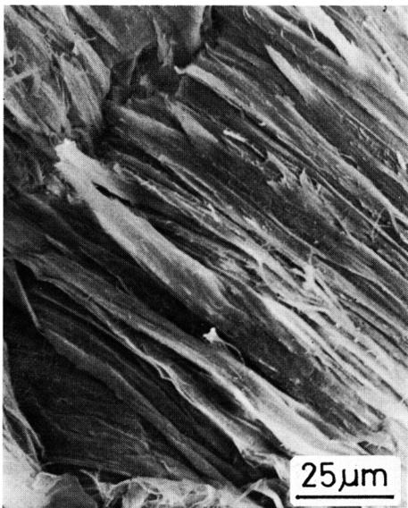
Photo 5. Thin-walled fibers in a radial phloem strand.
