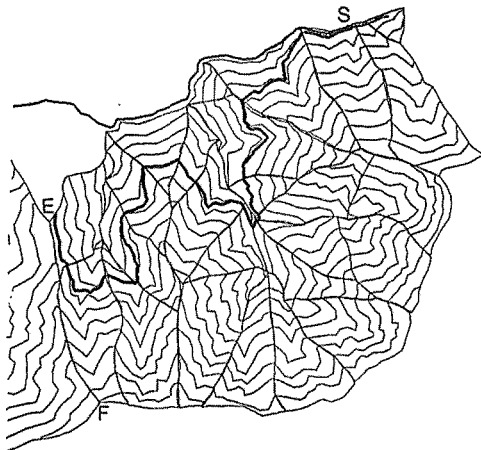
Fig. 3 Location of forest road on minimum cost of logging and road construction S: beginning point E-F: border line of end point
