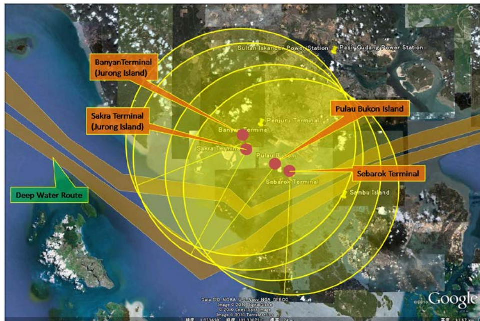
Fig. 4 Impact radius for toxic releases along the Singapore Strait. The yellow circles indicate the maximum distance to the toxic endpoint (e.g., chemicals including ammonia anhydrous, hydrogen sulfide anhydrous, hydrogen fluoride anhydrous). Prevailing winds will determine the direction of toxic plume hazard.
