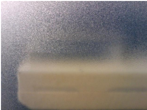
Figure 6: A picture of a block 1 cm away from a frosted glass board from a camera view.
