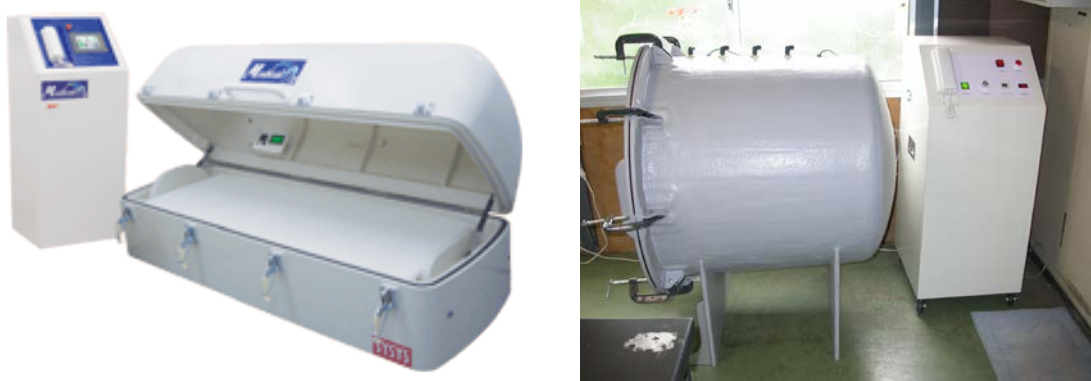
Fig. 1. Mild hyperbaric oxygen chambers for experimental animals (right) and humans (left). These chambers consist of an oxygen tank with an oxygen concentrator and an air compressor that automatically maintain an elevated atmospheric pressure and an increased oxygen concentration by using a computer-assisted system.
