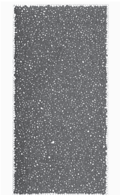
Fig.20 PFC model for the FLAC/PFC coupling analysis 54) . The model width is 0.5m and the height is 1.0 m.
