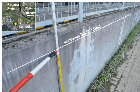
Photo 5 Inundation depth in the Kameoka city area (in front of Ion Kameoka store).
