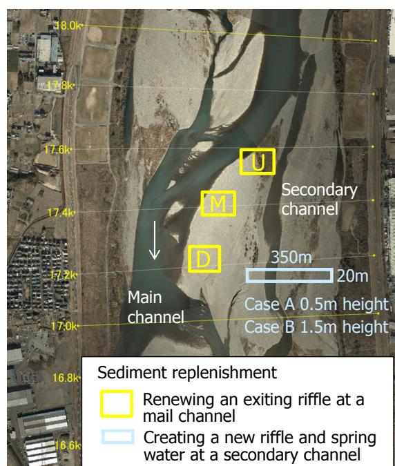
Fig. 13 Location and form of the replenished sediment for renewing an existing riffle at a main channel and for creating a new riffle and spring water at a secondary channel.
