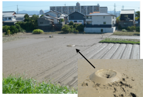
Photo 2 Sand volcano back of left bank of the Kamo river
