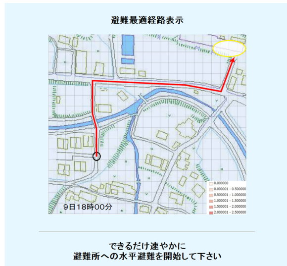
Fig.7 Inundation depth map (unit [m], 10m mesh) and optimal evacuation path : 0908091800[JST], at 2009 Sayou event
