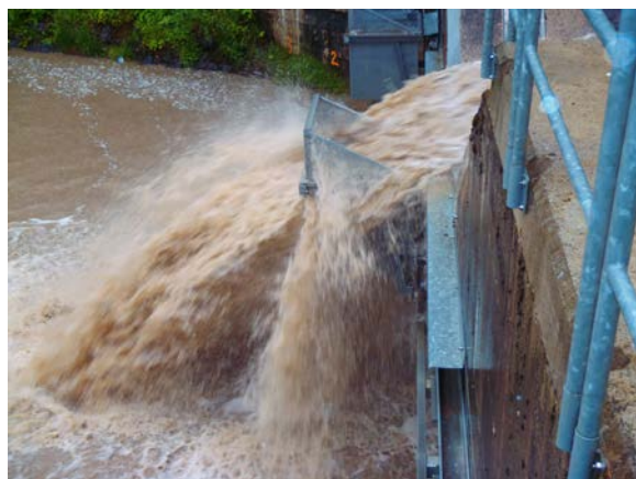
Photo 2 Bedload sampling by a moving basket at a rainfall event on July 29, 2013
