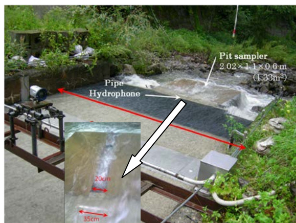
Fig. 2 A pipe hydrophone and a pit sampler at the Ashiarai-dani station
