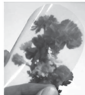
Figure 1. Wood pulp-based optically transparent nanocomposite.
