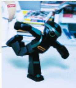
Humanoid robot, "Chroino." The robot is demonstrating a new biped walking technique called the "SHIN-Walk," which was developed by Robo Garage.
