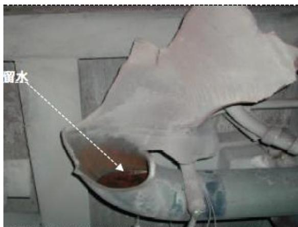
Fig. 1-1 A photograph of the ruptured pipe due to detonation of accumulated  $H_2$  and  $O_2$  at Hamaoka-1 nuclear power plant<sup>1)</sup>
