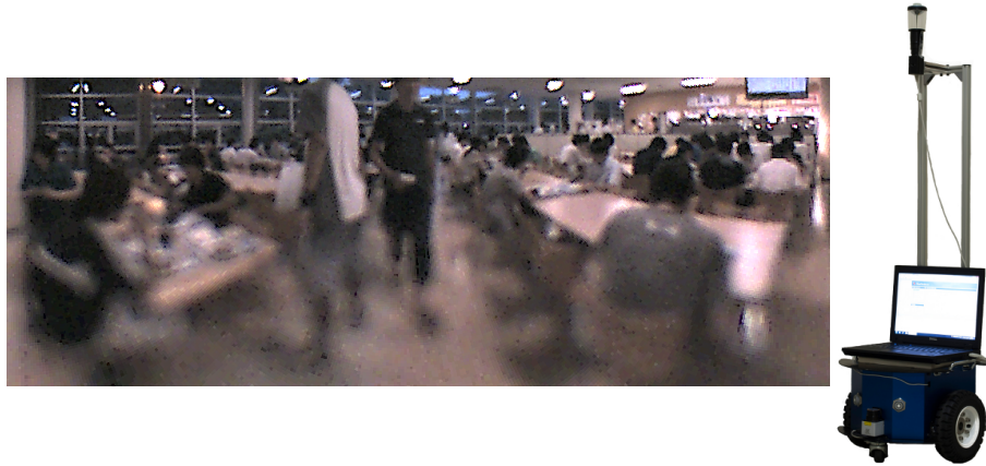
Fig. 5.2 The left image is an example of a crowded environment. This image was obtained by the robot in our experiment. Many people are constantly moving. The right image is the mobile robot used in this study. This robot has an omnidirectional camera at the top.
