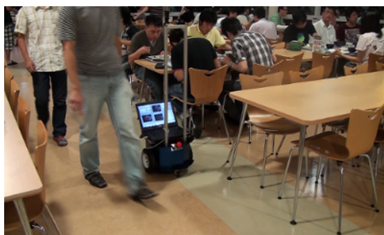
Fig. 5.11 The robot and the environment in the navigation phase. The robot could navigate autonomously in a crowded environment.
