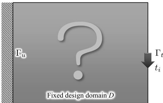
Fig. 5 Fixed design domain and boundary conditions of design model 1.
