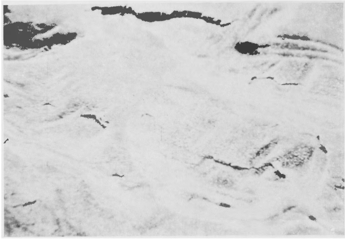
Fig. 14 A microscopic view (40X) of the mesh-side surface of a polyurethane diaphragm after six months of pumping. There are many cracks on the polyurethane surface.
