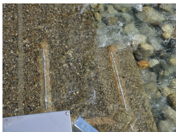
Fig. 1 Hydrophone installed on the Yodagiri river, Nagano, Japan (courtesy of T.Koshiba).
