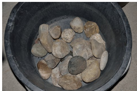
Fig. 6 Image of tested sediment stones of D_s = 100 \text{ mm} . (courtesy of T.Koshiba)
