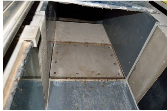
Fig. 3 Plate microphone in the test flume. Design similar to geophone system (courtesy of T.Koshiba).
