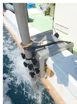
Fig. 7 Installation of Sonar to gunwale of the observation boat.
